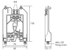
**SMB7 insulating mounting block** mounts on a flat surface and provides minimum overall installation height. Recommended maximum number of barriers between blocks is 25.
