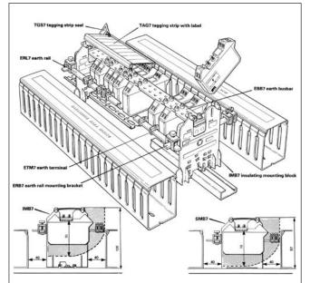
**End elevations with recommended spacing.** Shaded portions show areas swept by barrier during installation and removal.
